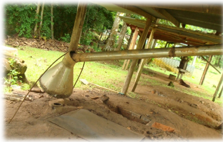
Image B6: The chimney of the Japanese oven
