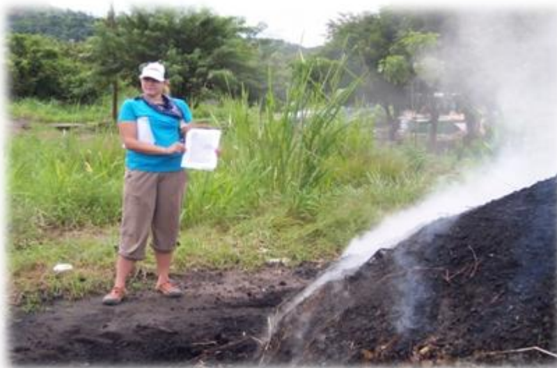
Image 8: Determining the smoke density by holding the smoke density chart next to the Traditional Oven
